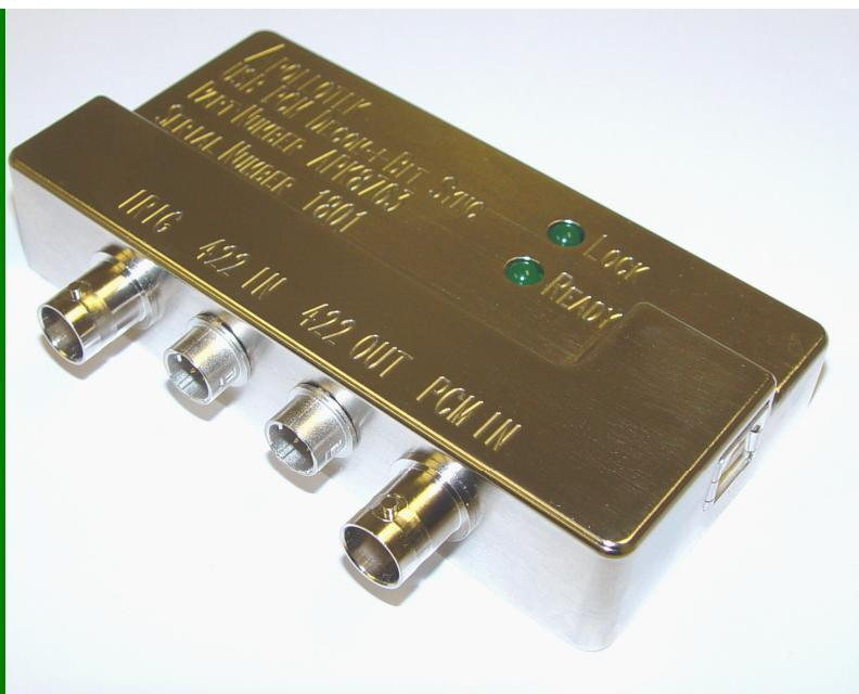
The Apollotek APK8763 Bit Synchroniser is part of the ApolloDas range of USB products which are designed for PCM Flight Test Instrumentation system checkout and test applications. The Unit is incorporated into an aerospace grade aluminium housing machined from solid which is rugged enough to be installed in an aircraft.
